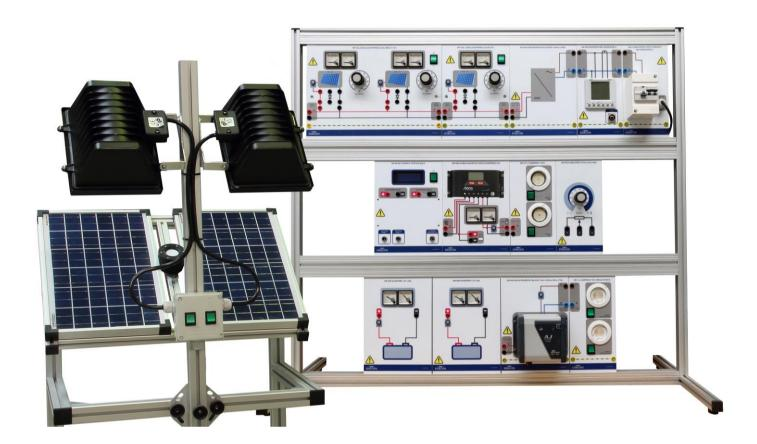
The equipment EN 01.5 reproduces a scale, complete photovoltaic solar installation. It has been designed with special emphasis on the didactic aspect. It offers the opportunity to observe all the components of a real photovoltaic solar installation and its layout.
